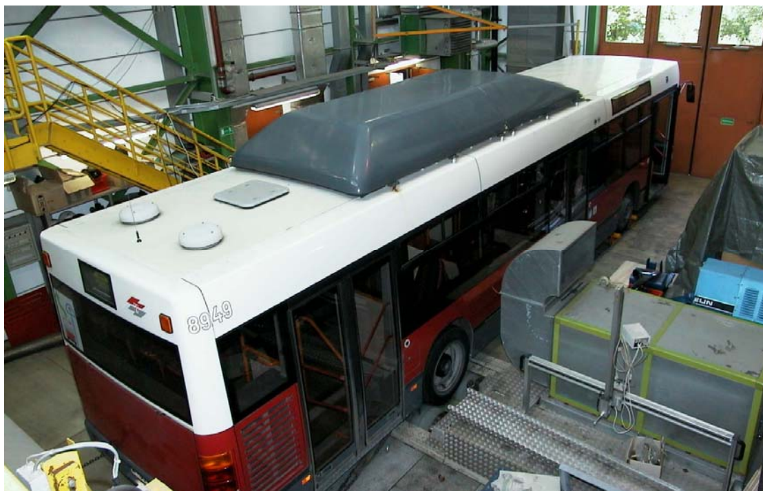
Figure 3: Transient roller test bed at TU-Graz for HDV up to 38 tons and 360 kW with full flow CVS system (CVS system not in the picture)
